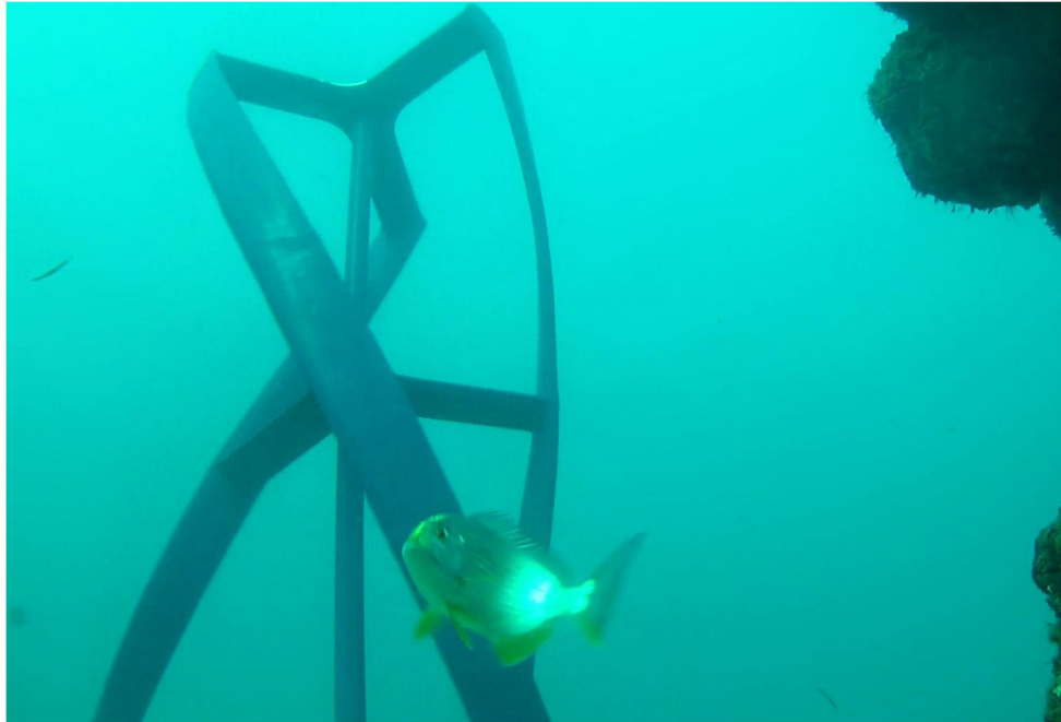
Figure 4. Example of Rhabdosargus sarba (F.) evasion manoeuvre. Goldline stumpnose R. sarba carrying out a typical evasion manoeuvre as the specimen passes through the gap against a 0.7 \text{ ms}^{-1} current speed. The fish changed its trajectory 45^\circ with a quick burst as it was startled by the approaching rotor blade at 22 cm distance. The image was extracted from the analysed video material (right camera).
