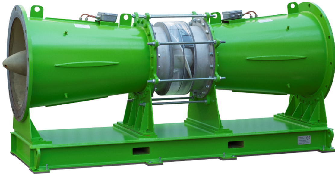
Figure 13. Pentair Fairbanks Nijhuis scale model turbine as tested in Maurik
